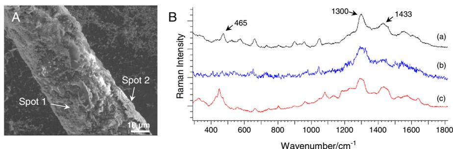
**Figure 2.** (A) SEM image of an alpaca fiber dyed with cochineal. (B) Stack of the SERS spectra measured in the SEM using SCA on the spot 1 (a) and 2 (b) shown in (A) and SERS spectrum of the reference sample of carminic acid obtained in the confocal optical microscope (c).
