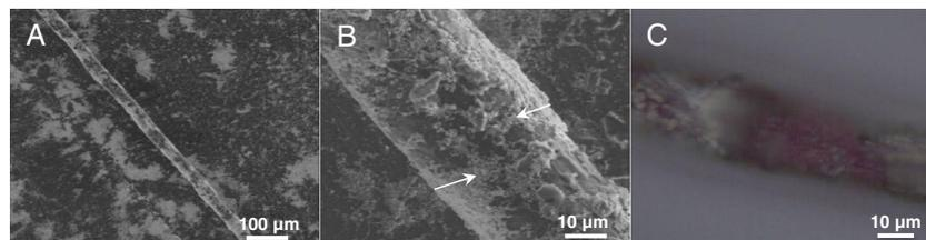
**Figure 1.** SEM (A, B) and light optical microscope (C) images of wool alpaca fiber with deposited silver nanoparticles. Arrows on the image B highlight the areas optimal for the  $\mu$ RS analysis. Those are not distinguishable on the optical micrograph, C.
