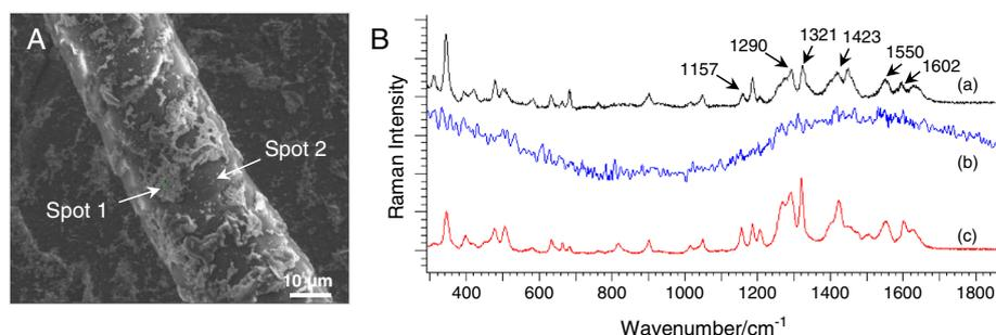
**Figure 3.** (A) SEM image of a wool fiber dyed with chay root. (B) Stack of the SERS spectra measured in the SEM using SCA on the spot 1, (a), and 2 (b) shown in (A) and SERS spectrum of the reference sample of alizarin obtained using the confocal optical microscope (c).
