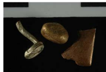
Figure 8. Objects 2A, 2B, and 2C, showing differences in colour due to different proportions of gold, silver, and copper.
