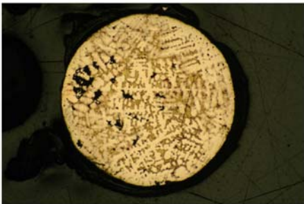
Figure 6A. Polished and etched cross-section of sample 2A, showing that this wire was cast to shape, without further modifications.
